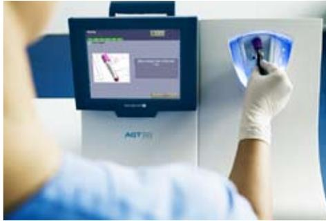
Place the closed sample directly into the inlet. No sample preparation is required.
