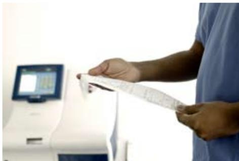
After 30 seconds, the AQT90 FLEX analyzer is ready for the second sample. Results are printed and sent to the LIS/HIS or directly to patient monitors.
